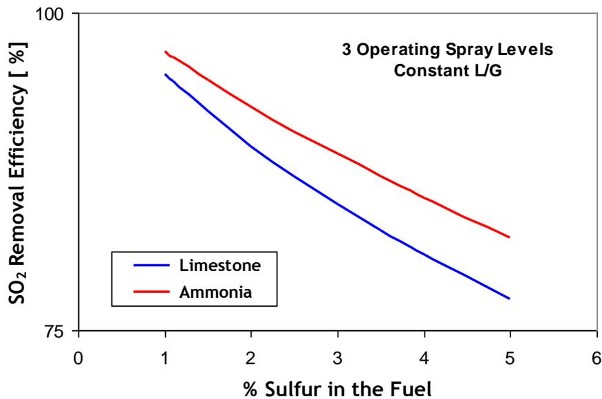
*Figure 2 – Impact of Fuel %S on SO<sub>2</sub> Removal for Ammonia versus Limestone*
